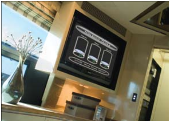
With the push of a button, TechLink tracks the status of batteries, fluid levels, and temperatures throughout the coach and displays them on the dash, bay, and all television monitors.
