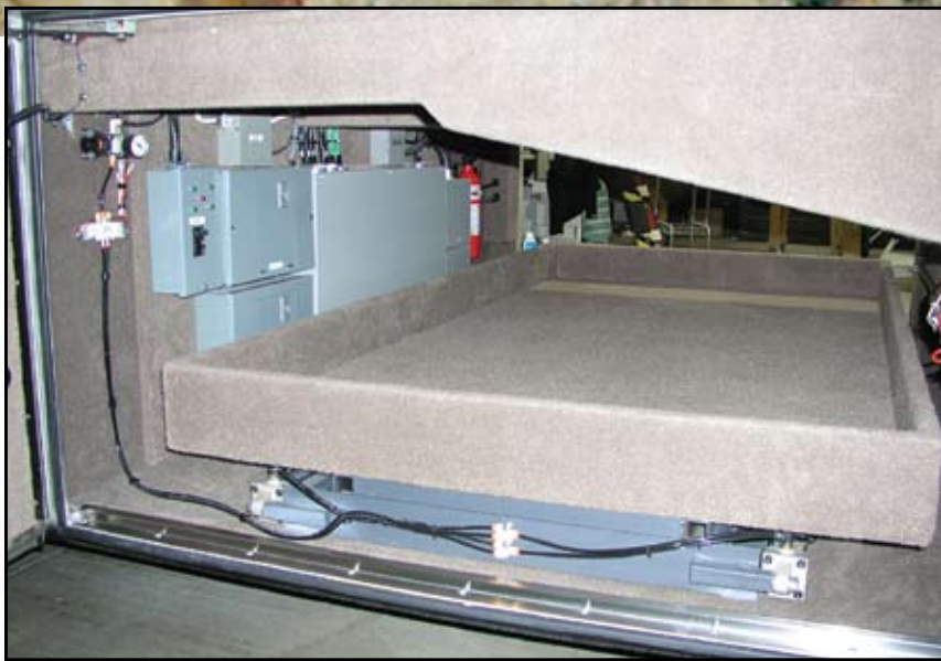
Slide-masters have a 2,000-pound capacity and pull out like a huge drawer.
