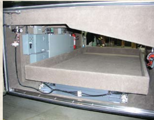
Slide-masters have a 2,000-pound capacity and pull out like a huge drawer.
