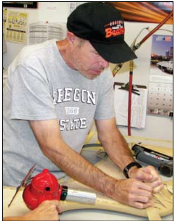
An industrial blow-dryer makes stiff leather more malleable for Will Wood to stretch it taut across the door panel before stapling it down.
